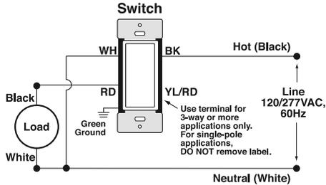
**THREE-WAY WIRING DIAGRAM**
