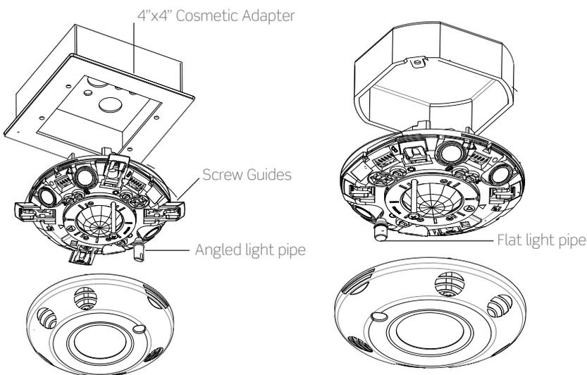
Sensors conveniently mount to a standard 4" x 4" square or octagon electrical box per NEC standards
