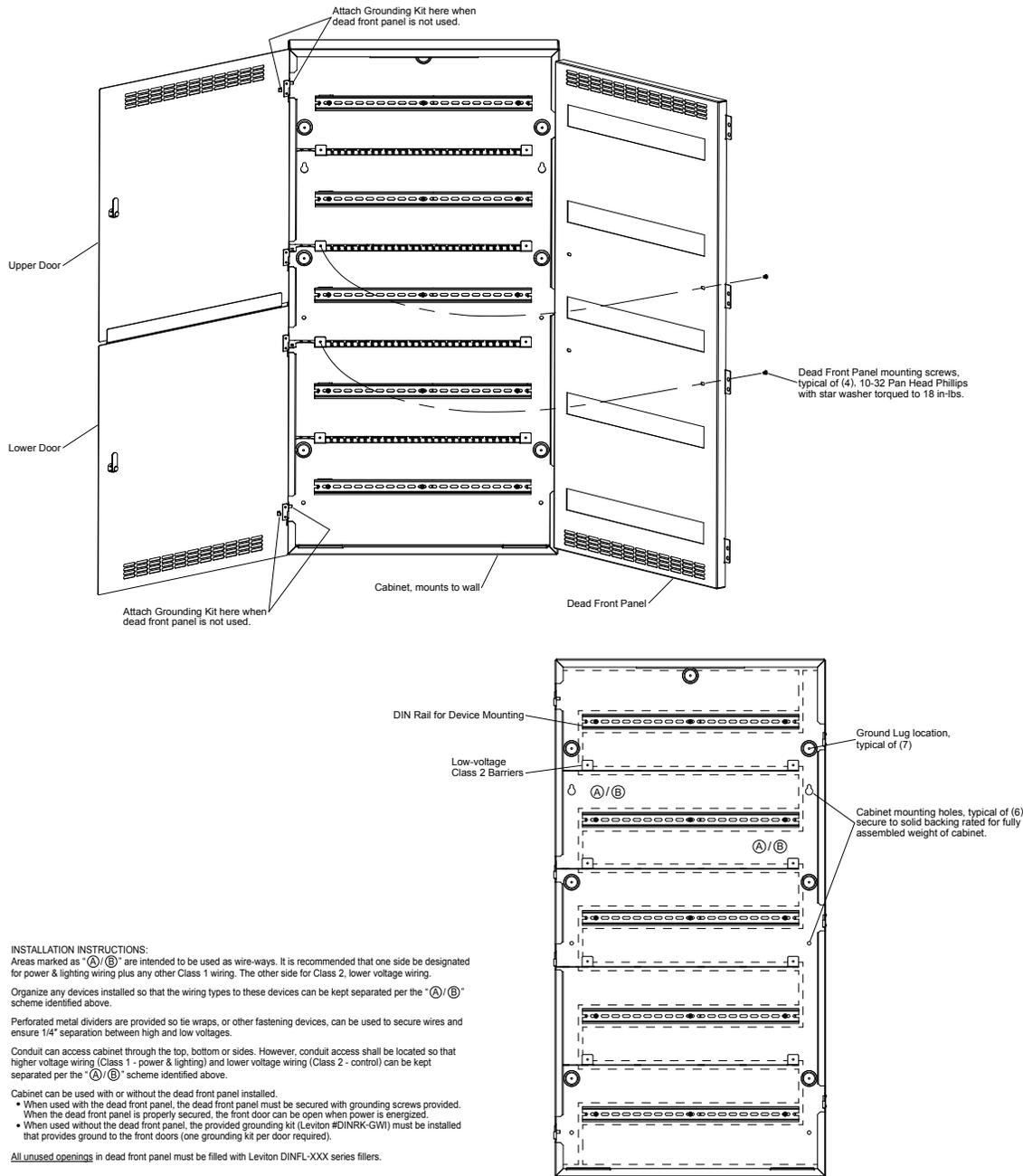
Areas marked as “(A)/(B)” are intended to be used as wire-ways. It is recommended that one side be designated for power and lighting wiring plus any other Class 1 wiring. The other side for Class 2, lower voltage wiring.
