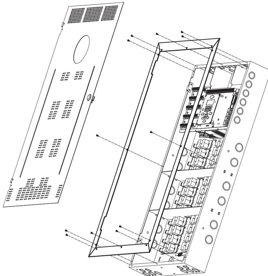
**Figure 2: Flush Kit Mounting Pictorial (24 relay cabinet shown, other similar)**
