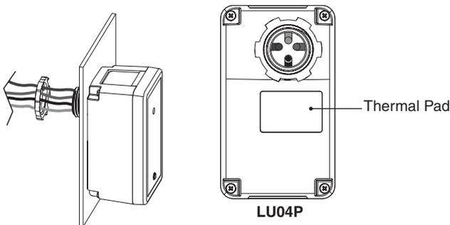
2. Strip wires 3/4 in and connect as per wiring diagram. Ensure wires are firmly attached and there is no exposed copper.
