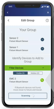
• Select Magnifying Glass icon of the sensor you would like to add; the light with attached sensor will blink to indicate the sensor has been selected
