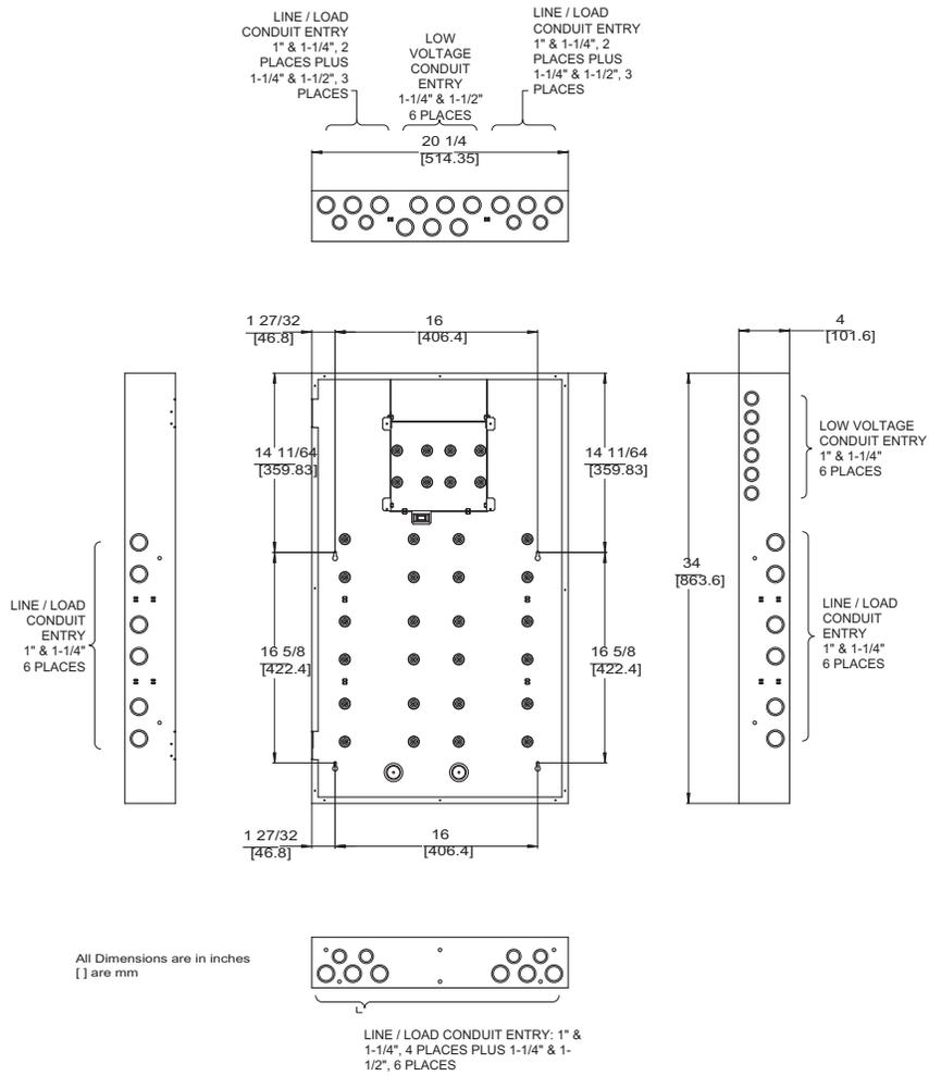
**Figure 5: EZ-MAX Plus 16/24 relay cabinet mounting provisions and dimensions.**
