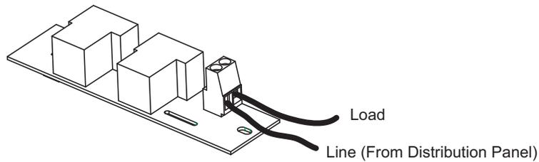
**Figure 9: Wiring Diagram for EZ-MAX Plus 1 Pole Relay Card (latching relay card similar)**
