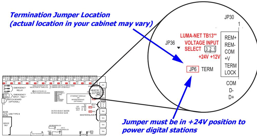
**Figure 21: Typical termination jumper location**
