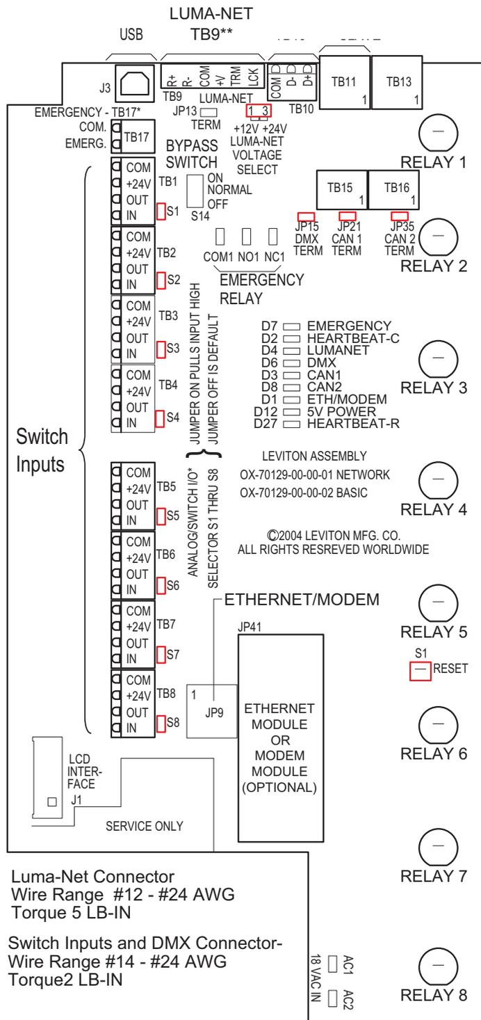
**Figure 17: Inside layout of an EZ-MAX 8-Relay Cabinet.**
