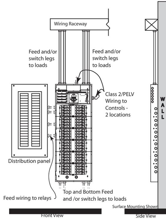
**Figure 3: Sample Electrical Room Layouts for all cabinets**
