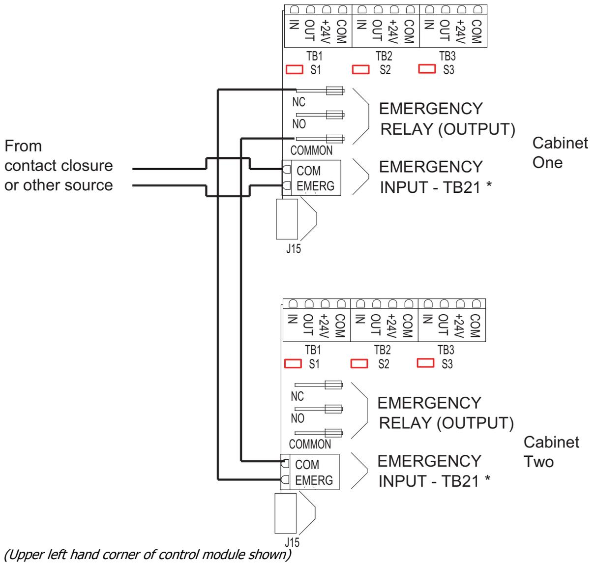
**Figure 23: Wiring Diagram for 16/24 relay cabinets showing (2) interconnected Emergency Cabinets.**
