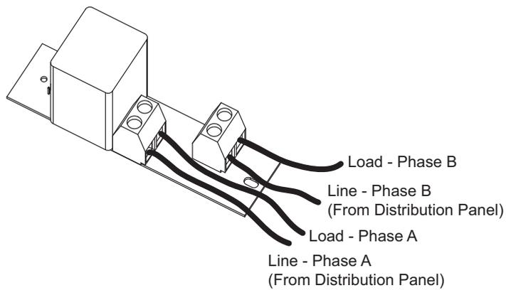
**Figure 10: Wiring Diagram for 2-Pole Relay Card**
