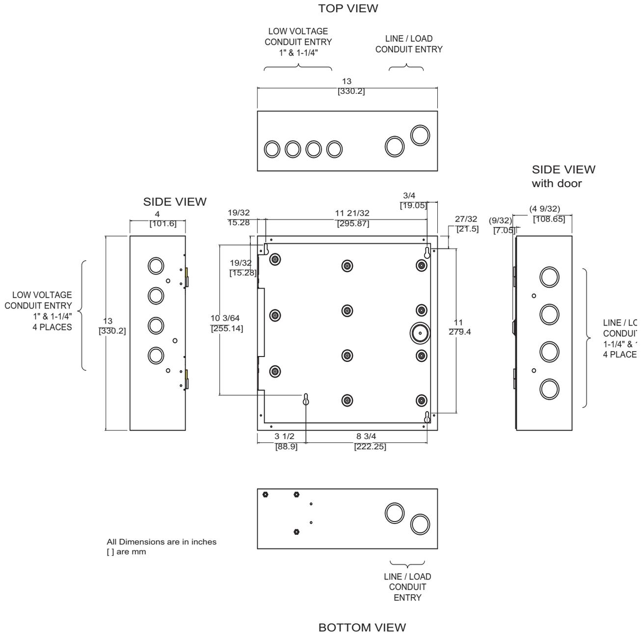
**Figure 4: EZ-Max Plus 8 Cabinet mounting provisions and dimensions.**
