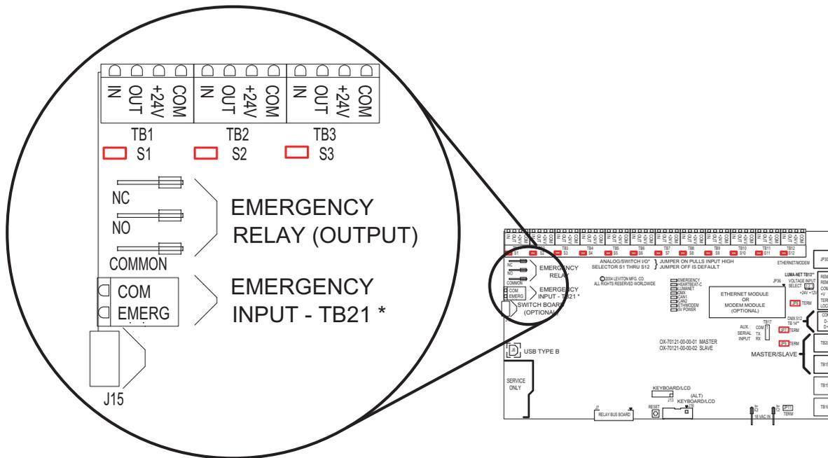
Figure 22: Emergency Input and Output Connectors 16/24 relay cabinets
