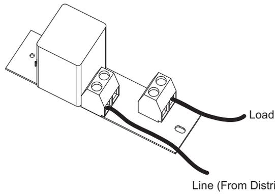
**Figure 11: Wiring Diagram for EZ-Max Plus 347 V Relay Card**
