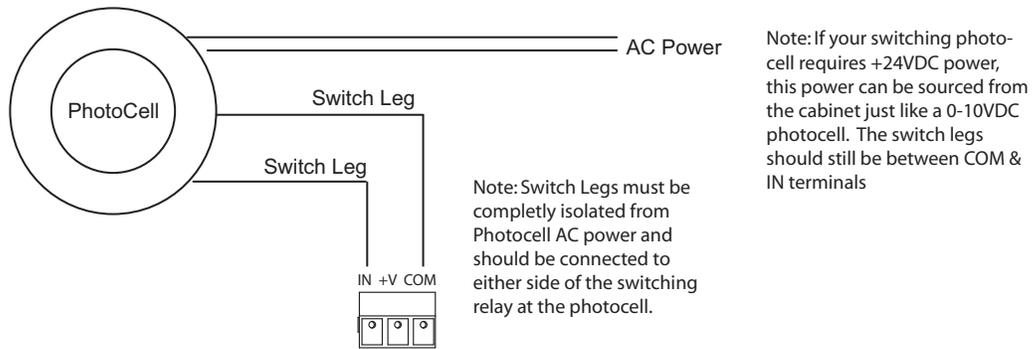
**Figure 20: Switching Photocell**
