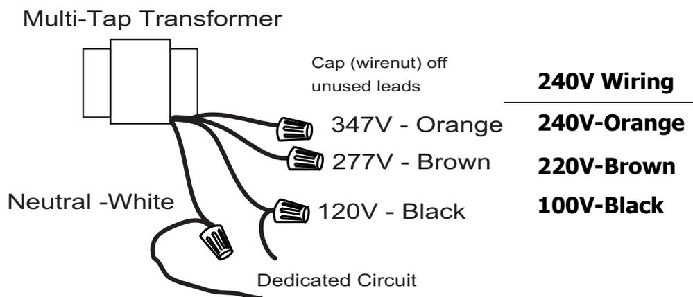
**Figure 13: EZ-MAX Plus 16/24 Relay Cabinets Control Electronics Power**
