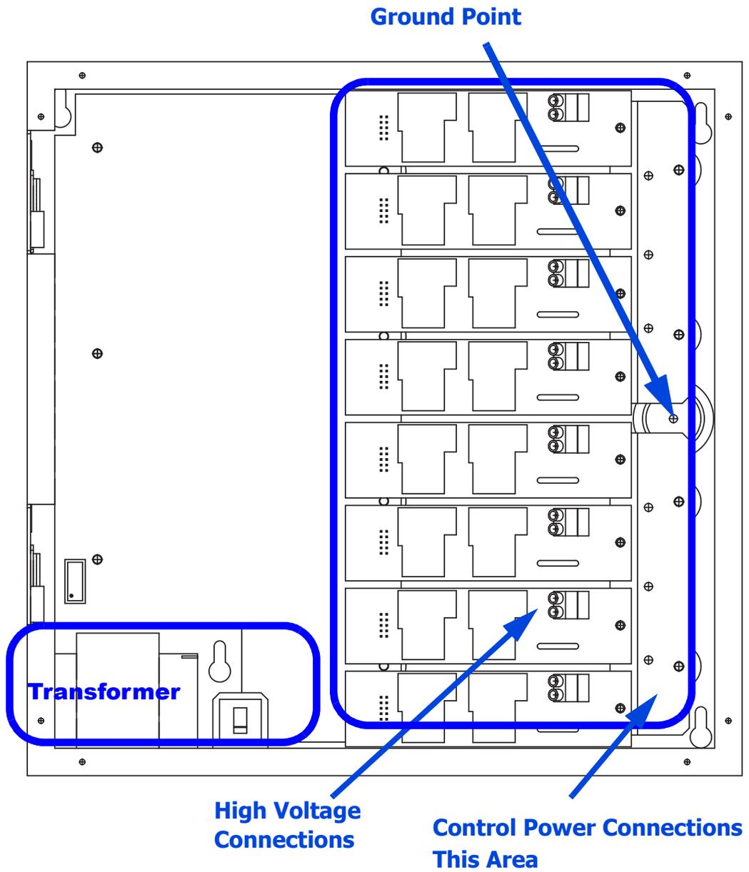
**Figure 6: EZ-MAX Plus 8 Line Voltage Wiring Areas.**
