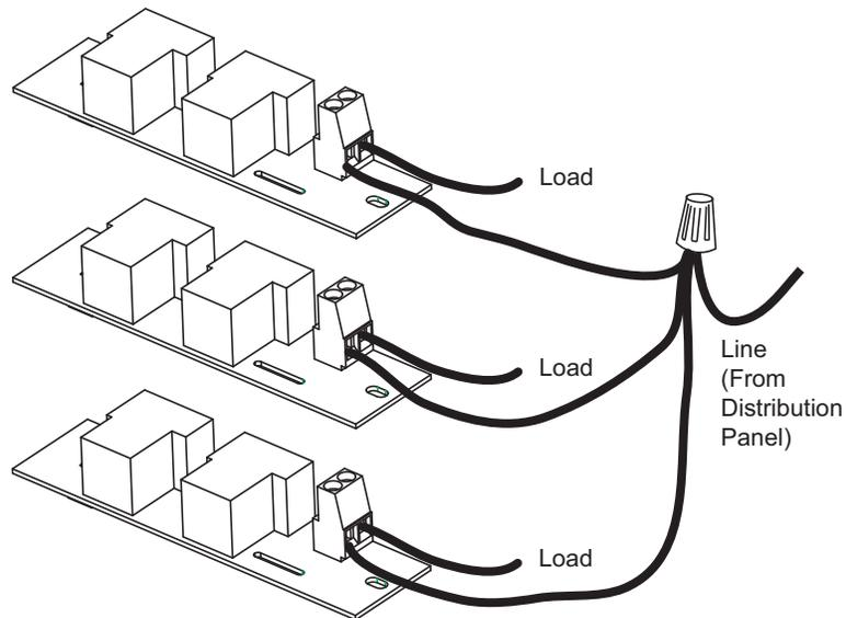
**Figure 12: Wiring of Multiple Relays to Common Branch Circuit Breaker**
