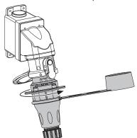
3. Fully insert plug into receptacle until it latches with the spring-loaded pawl.
