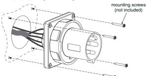
If mounting to a backbox, use Leviton: BX60LEV (60A/63A), BX100LEV (100A/125A) - non-metallic BX60LEVM (60A/63A), BX100LEVM (100A-125A) - metallic
