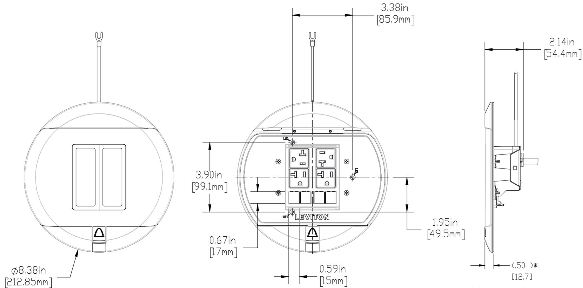
NOTE: ABOVE VIEW DENOTES ELECTRICAL / RECEPTICAL OPENINGS. EXTERIOR LID REMOVED FOR CLARITY.
